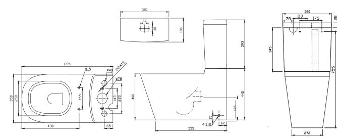
Universal set out 95mm to 200mm P/trap set out 185mm Recommended set out 140mm 784
